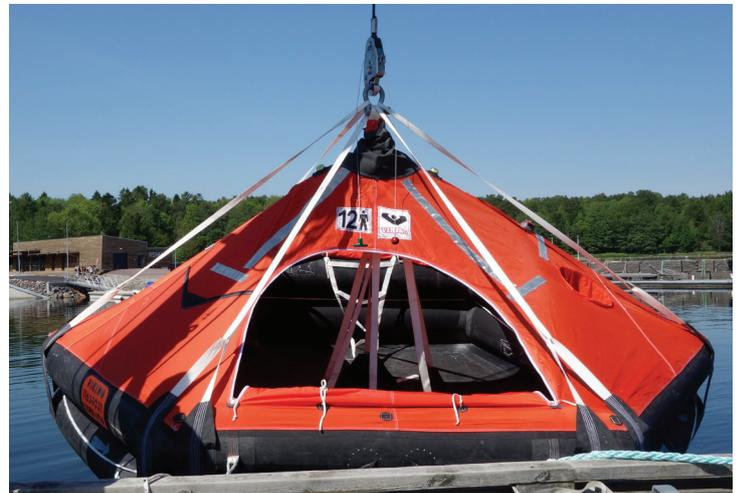
If conditions are such that it is not possible to use the automatic release capability, the Henriksen Liferaft Hook also offers a manual opening facility. It can be used if the raft is on the water but is being pulled by a strong current or by vessel movement and the automatic release capacity is not enough. Under these circumstances, a green grip on the hook can be pulled strongly and the hook will open.
